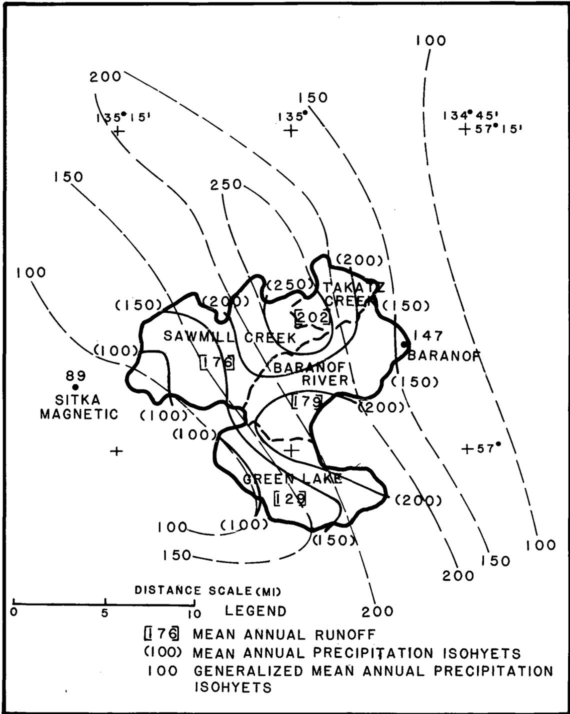
Figure 10.—Analysis of mean annual precipitation (inches) with adjoining basin runoff as input.
