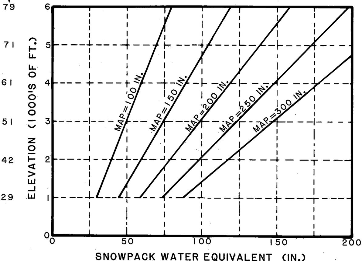
Figure 8.—Variation of snowpack water equivalent with elevation and mean annual precipitation.
