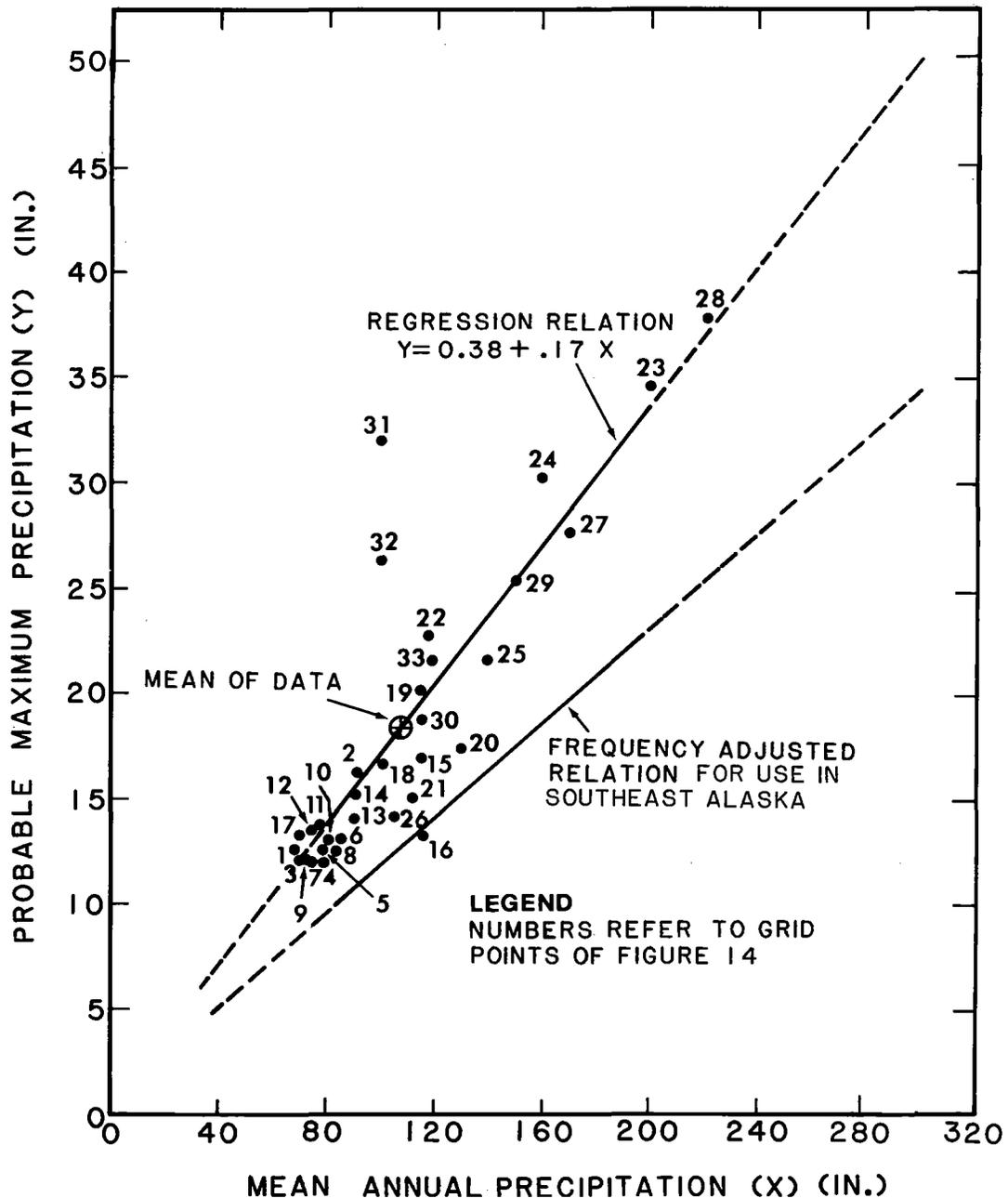
Figure 15.—24-hr 10-mi<sup>2</sup> probable maximum precipitation vs. mean annual precipitation from western Washington data.
