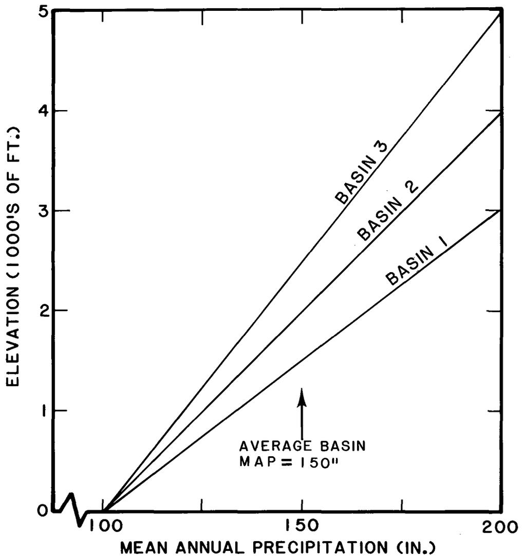
**Figure 38.**--Schematic for illustrating how mean annual precipitation variation can be determined for use in snowpack accumulations when mean annual precipitation  $\geq$  150 in. (3810 mm).
