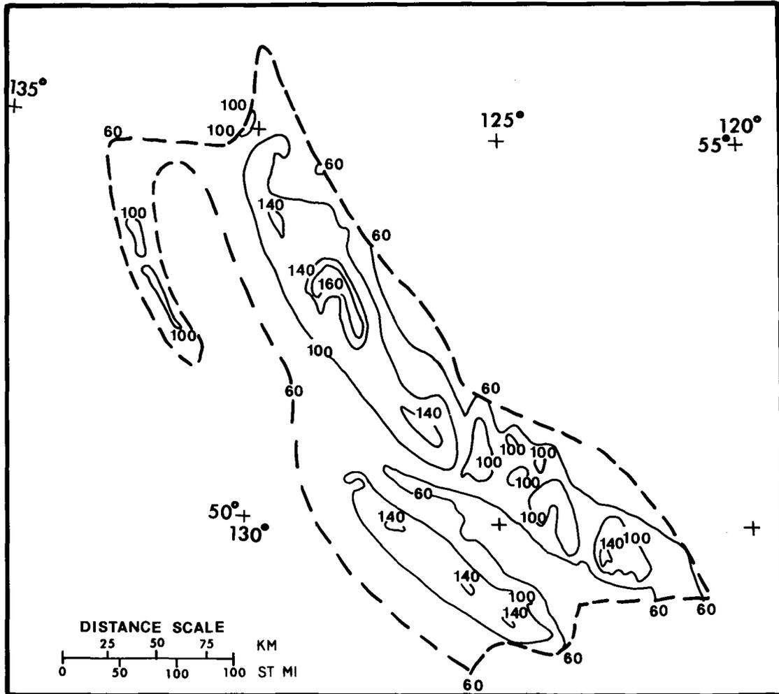
**Figure 20.—Area in British Columbia used for determining average orographic effects (after Walker, 1961). Isolines are mean annual precipitation in inches.**
