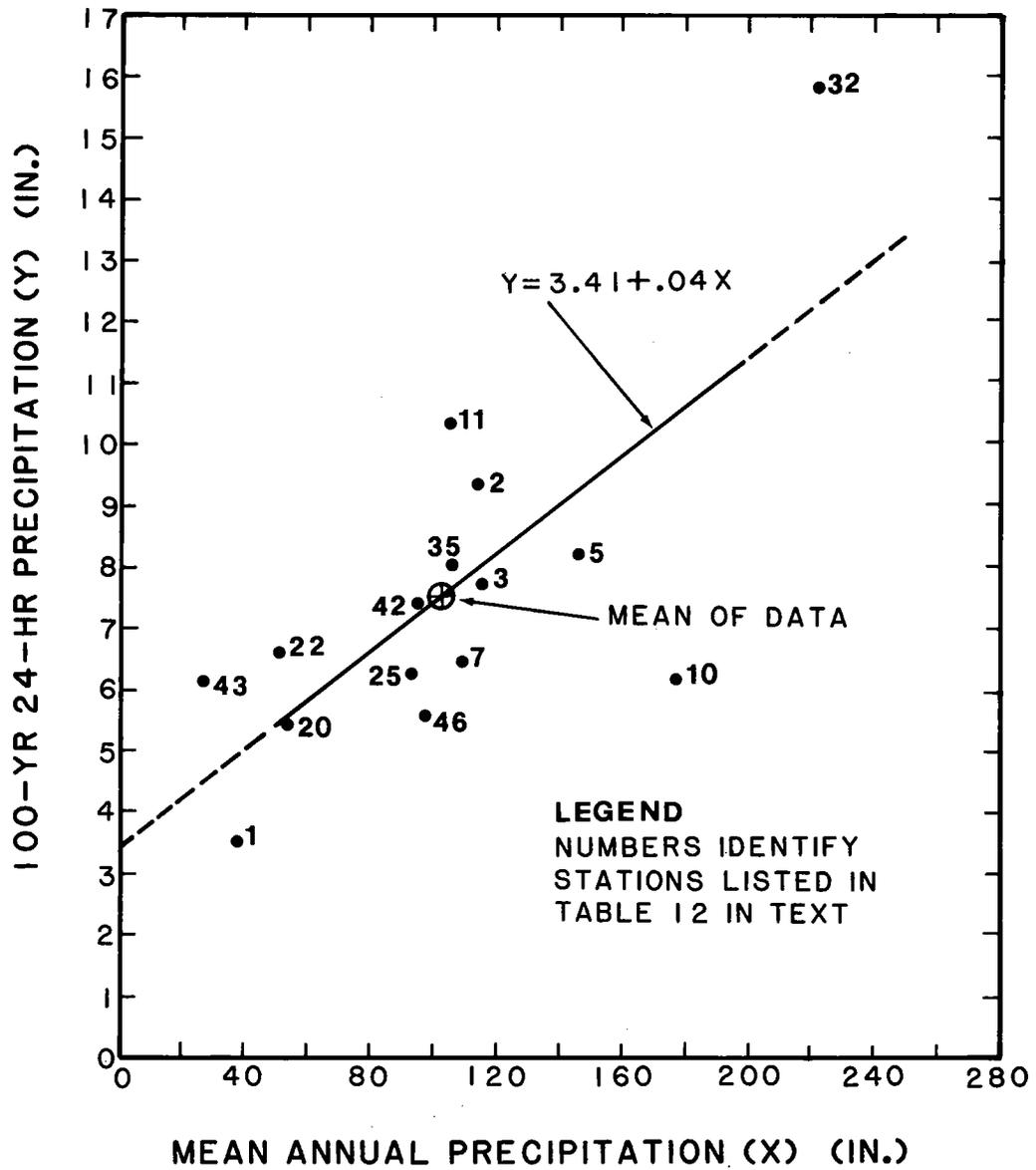
Figure 17.—100-yr, 24-hr precipitation vs. mean annual precipitation for southeast Alaska data.
