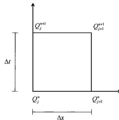
FIG. 1. Schematic of  $x$ - $t$  Plane for Muskingum-Cunge Model
