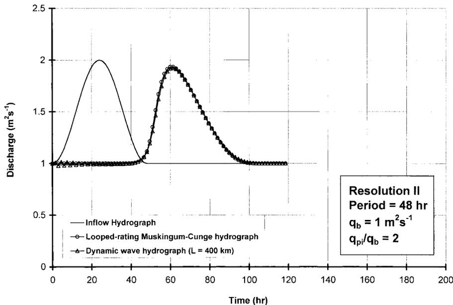
FIG. 4. Comparison of Outflow Hydrographs Generated by the Looped Rating Muskingum-Cunge and Dynamic Wave Models at a Distance of 200 km
