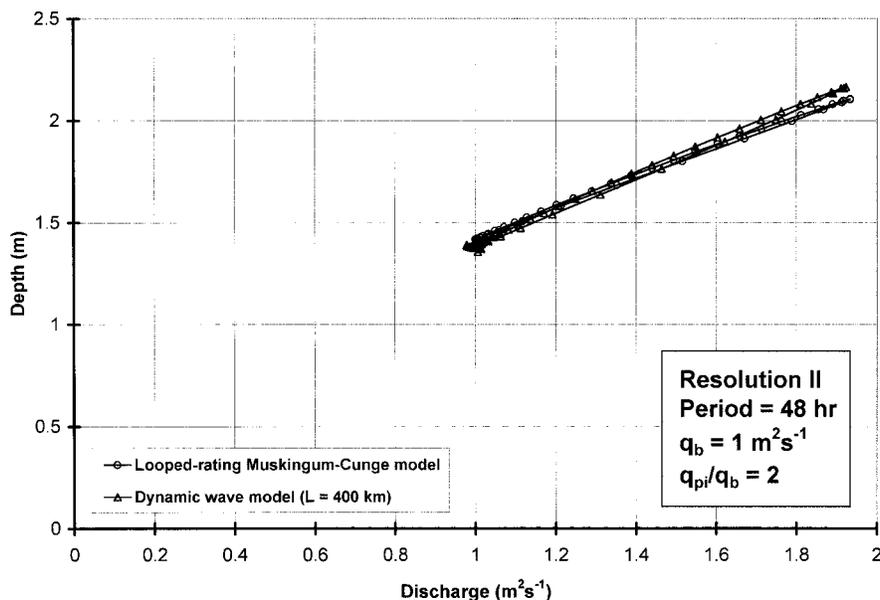
FIG. 3(a). Typical Looped Ratings Generated by the Muskingum-Cunge and Dynamic Wave Models at a Distance of 200 km— $L = 400 \text{ km}$
