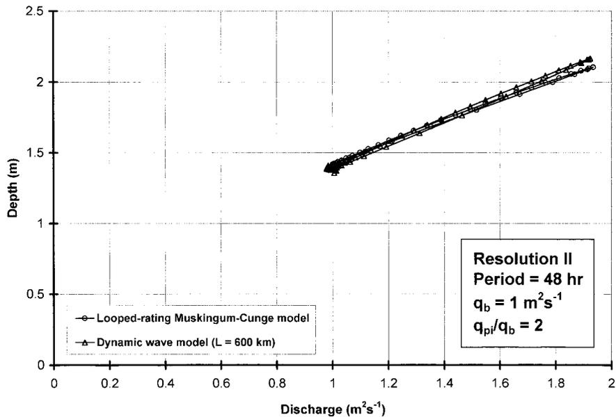
FIG. 3(b). Typical Looped Ratings Generated by the Muskingum-Cunge and Dynamic Wave Models at a Distance of 200 km— $L = 600$  km
