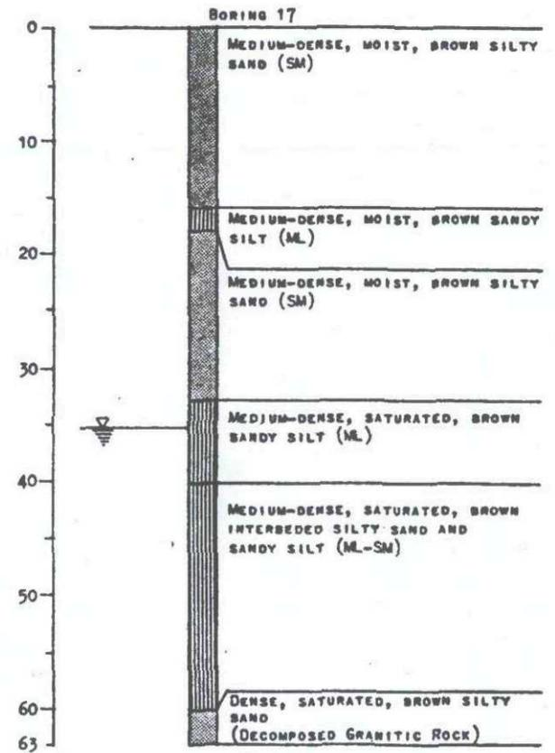
LOGS OF TEST BORINGS 15 THRU 18
