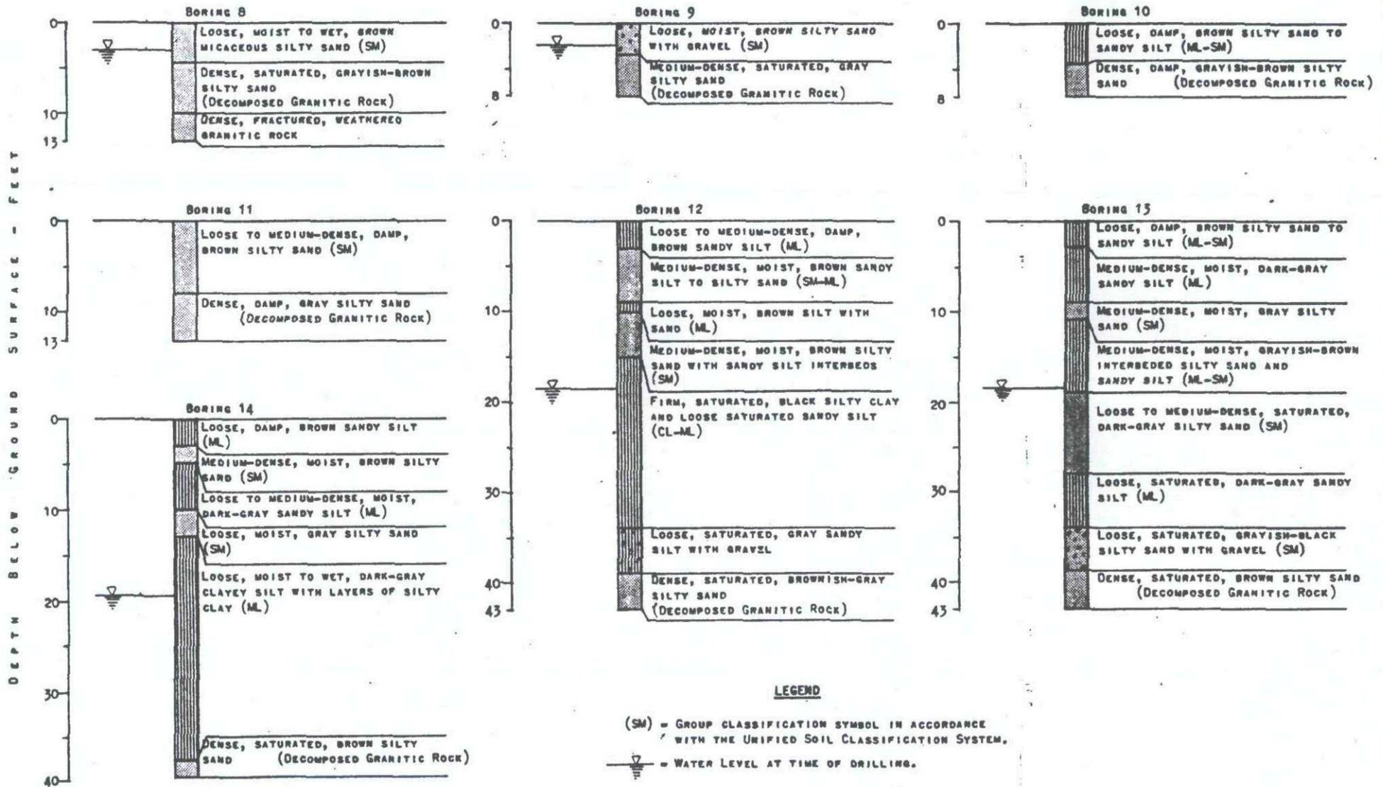
LOGS OF TEST BORINGS 8 THRU 14
