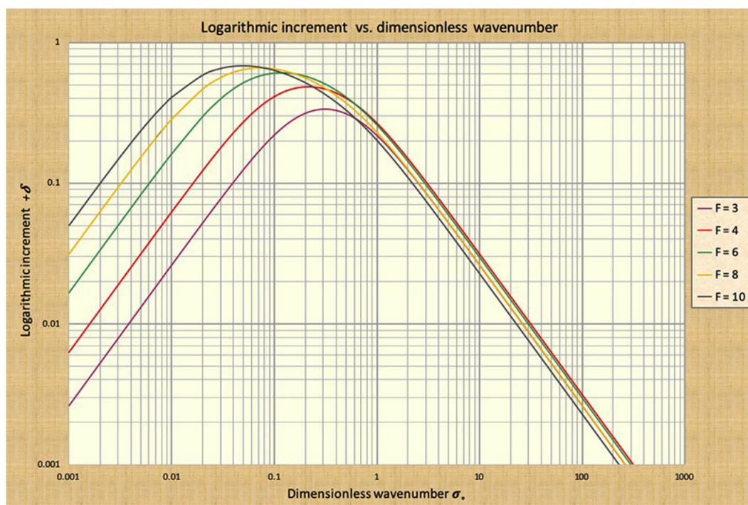
Fig. 3 Logarithmic increment  $+\delta$  vs dimensionless wavenumber  $\sigma_*$  for  $F > 2$ .
