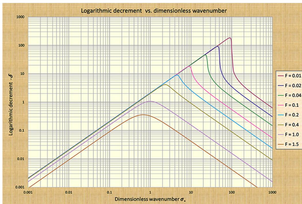
Fig. 2 Logarithmic decrement  $-\delta$  vs dimensionless wavenumber  $\sigma_*$  for  $F < 2$ .
