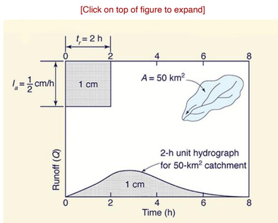
Fig. 2 (a) The unit hydrograph.
